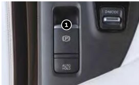
To apply the parking brake, pull the electric parking brake switch ① up, located below the instrument panel, regardless of the ignition switch position.
