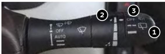
Move the lever (1) up or down to one of the following positions to operate the windshield wipers:
