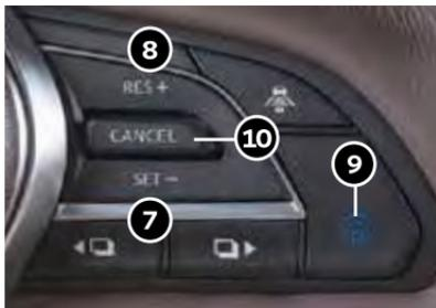
To set ProPILOT Assist, press the ProPILOT Assist switch ⑨ on the steering wheel. The ProPILOT Assist status ④ will appear on the vehicle information display. When the desired cruising speed is reached push the **SET-** switch ⑦ and release it.
