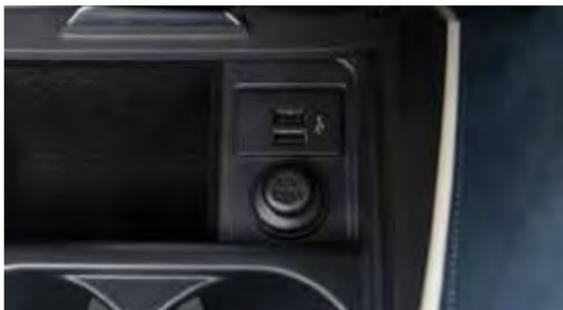
Your vehicle is equipped with two USB ports, located under the control panel, to which you can connect compatible devices (cellular phones, iPods, other compatible audio devices, USB memory sticks, etc.).
